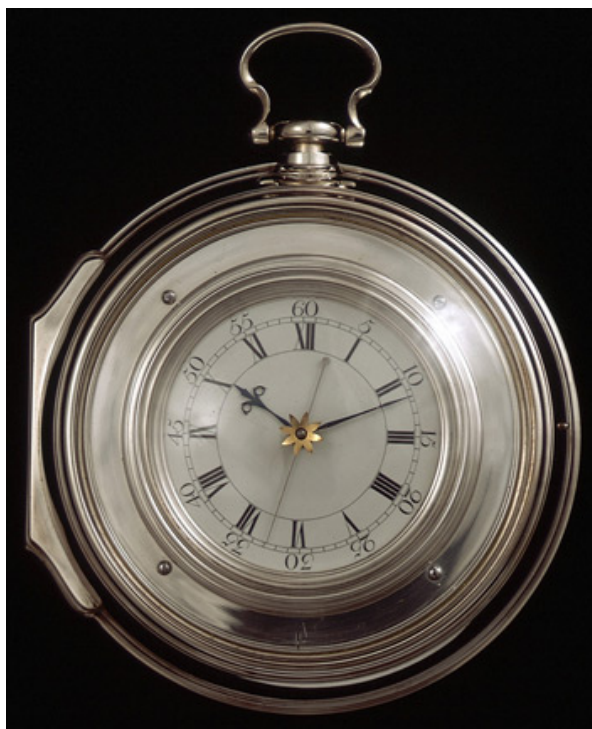
H5. Visually simpler in design than H4, H5 was of very similar technical construction. The watch was tested, with great success, by King George III at his private observatory in 1772. (Clockmakers’ Company. NMM ref: D6768)
