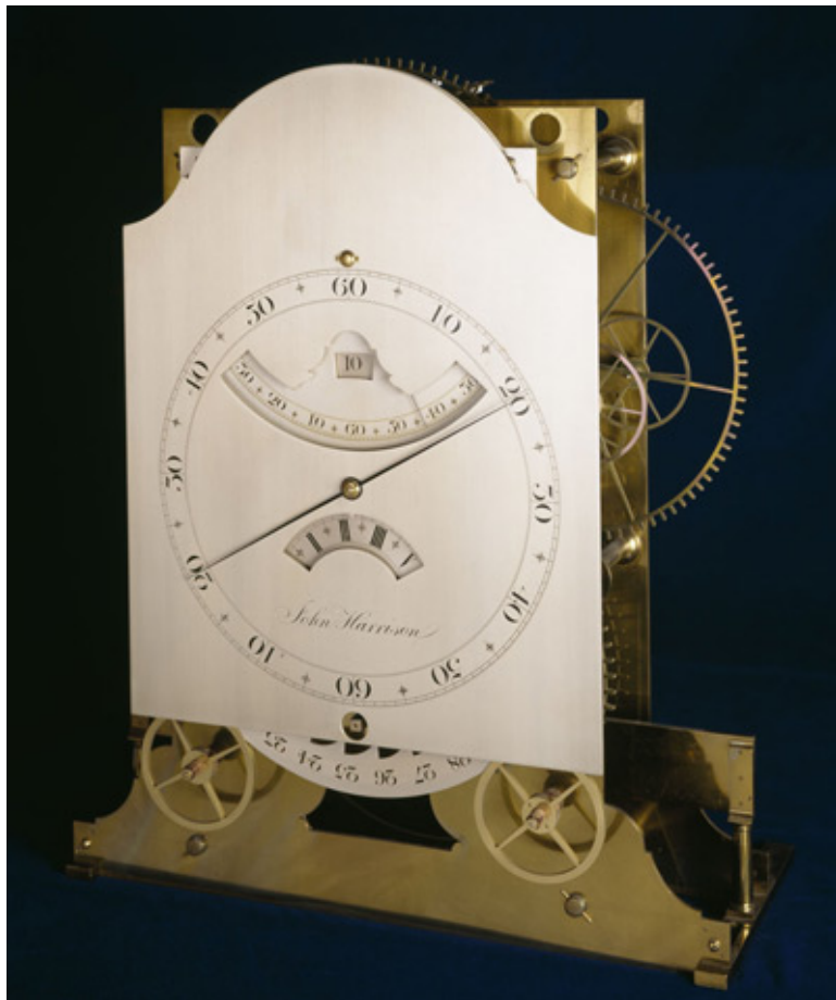
John Harrison's 'RAS' regulator. Built approximately in parallel with H3, this was Harrison's 'state of the art' fixed pendulum clock. He claimed timekeeping as good as a second in one hundred days from it (NMM ref: D6786-1).
