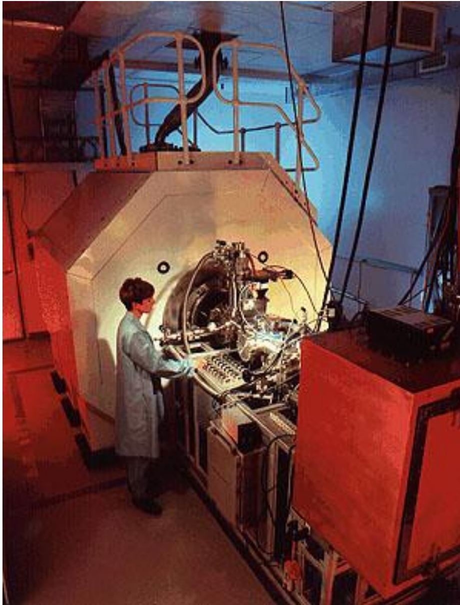
Thermo Finnigan FT ICR (Ion cyclotron resonance) 11.5 Tesla Massenspektrometer
