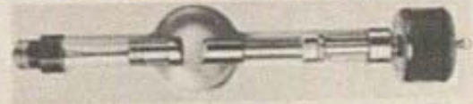
Fig. 25. Maclett bulb-type tube, more simple in construction and cheaper in price; available in 1.5 mm., 2-5 mm., 3-2 mm., and 3-8 mm., and in one double focus combination.
