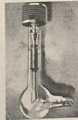
Fig. 28. For dental work a "right-angle" tube has been constructed. The outside side of this tube is grounded and the tube can be placed close to the patient's face.
