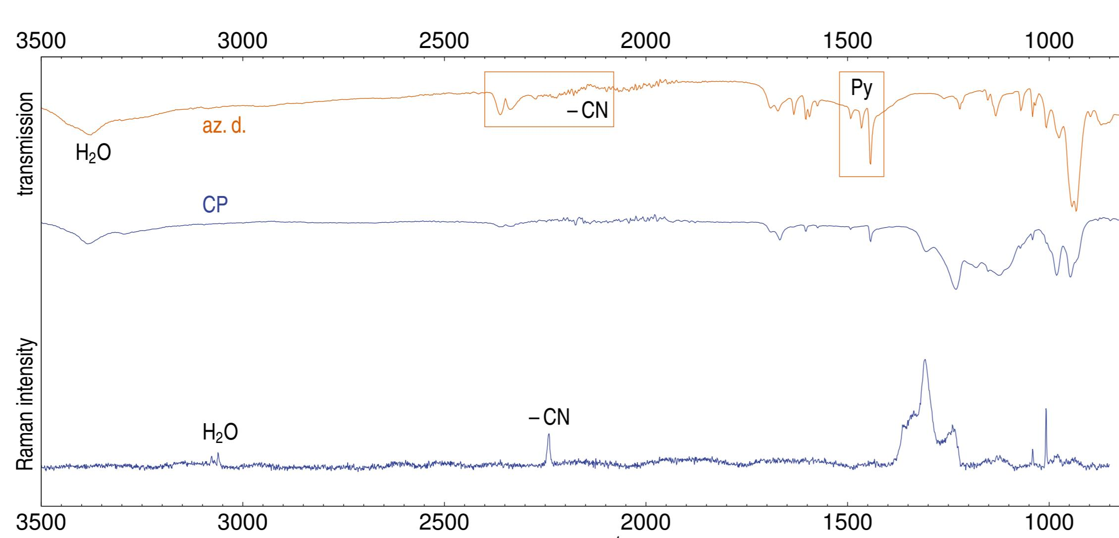
Fig. 3: Infrared and Raman spectrum of  $[\text{Mg}(\text{H}_2\text{O})_4(\text{Py})_2]\text{[B}(\text{CN})_4\text{]}_2 \cdot \text{H}_2\text{O}$  obtained through a crystallization preparation (CP) and by azeotropic distillation (az. d.), respectively.
