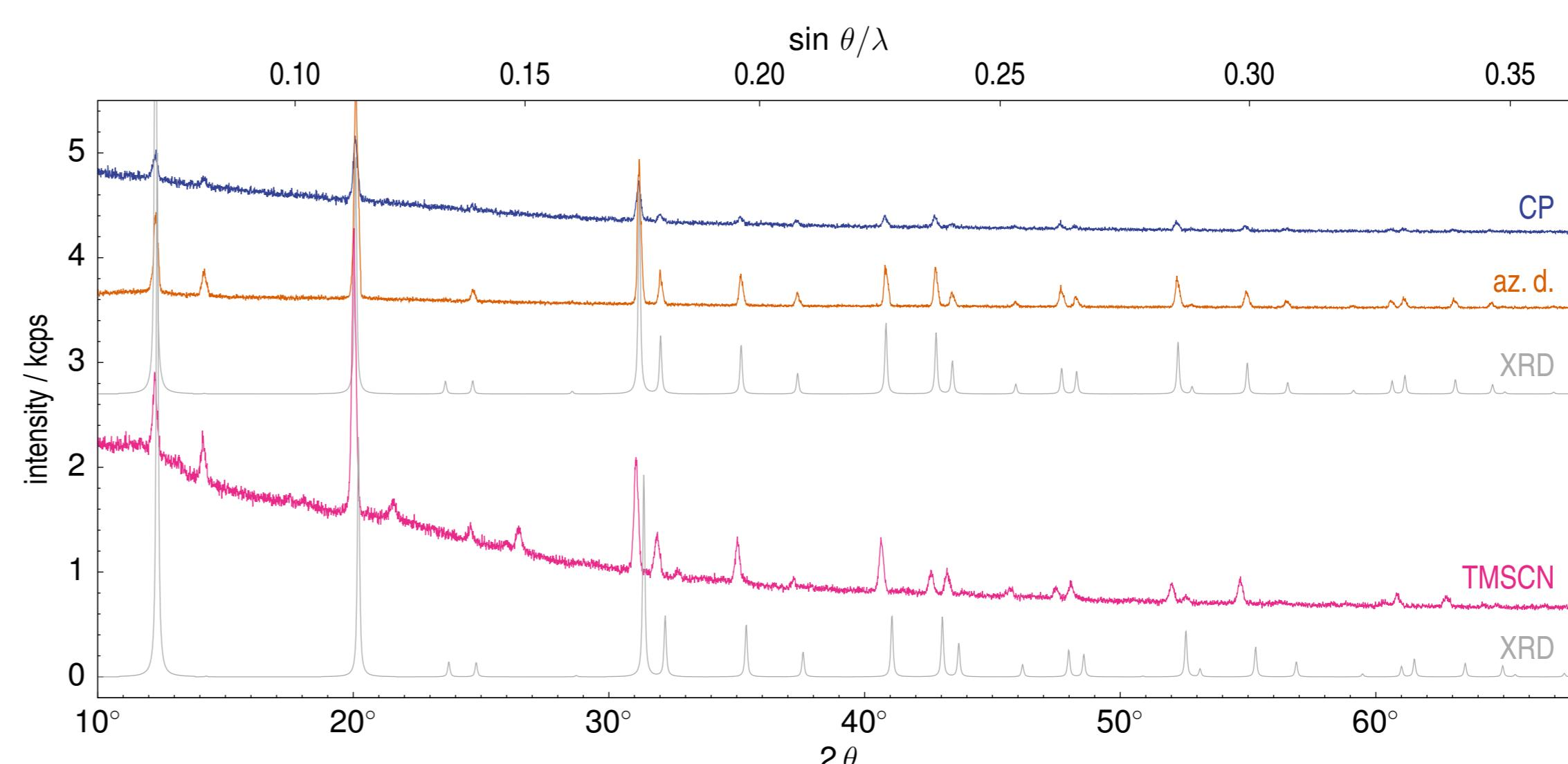
Fig. 2: X-ray powder diffraction patterns of  $\text{Sr}[\text{B}(\text{CN})_4]_2$  obtained by different methods: crystallization preparation (CP), azeotropic distillation (az. d.), calculated pattern from XRD dataset solved in  $F\bar{m}\bar{3}m$ , and drying with TMSCN: powder and calculated pattern from crystal;  $\lambda = 154.06 \text{ pm}$  (Cu).
