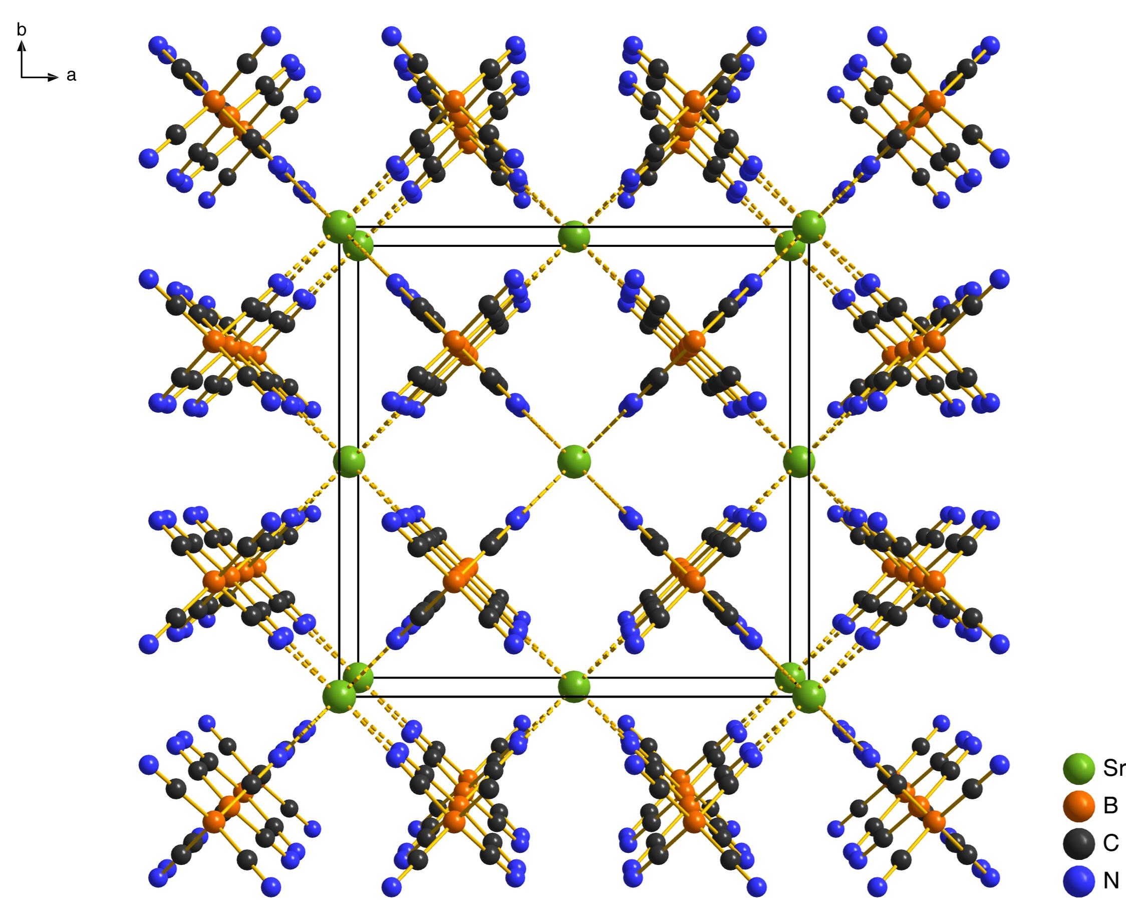
Fig. 1: View of the cubic structure of  $\text{Sr}[\text{B}(\text{CN})_4]_2$  along the  $c$  axis.
