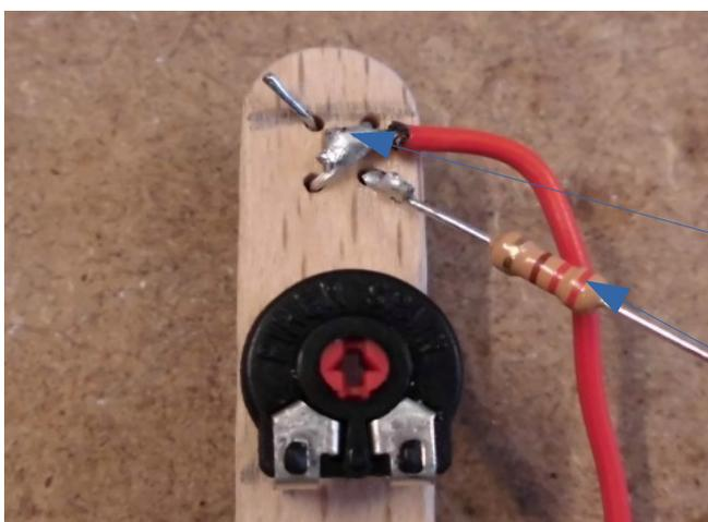
A red wire should be soldered additionally.
