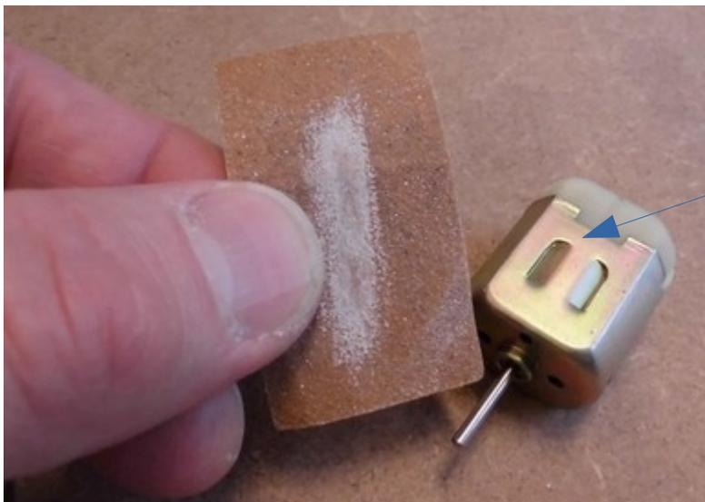
Grind the unprinted side!
