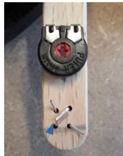
Two „legs“ of the photocoupler must be bent together and soldered.
