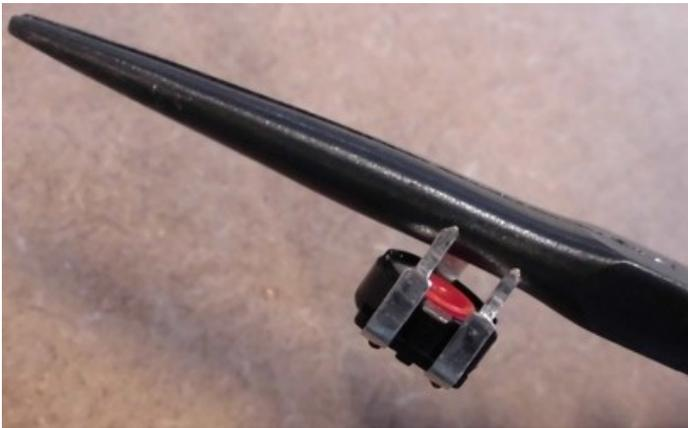
→ The „legs“ of the adjustable resistor should be bent straight.
