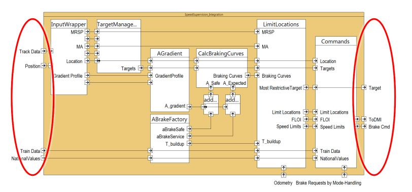
ANSYS<sup>®</sup> SCADE System view of SDM (simplified)
