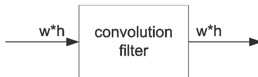
Figure 10: SDF model of a convolution filter. w is the image width, h the image height. Each output pixel depends from the local neighbor pixels belonging to the sliding window and can for instance be calculated by Equation (5).
