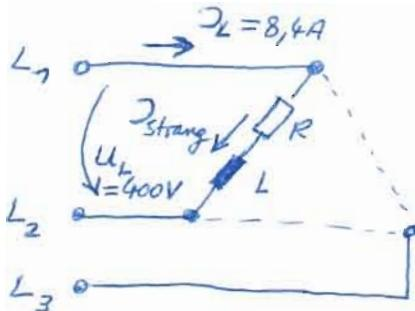
$$\underline{\underline{I_{\text{Strang}}} = \frac{I_L}{\sqrt{3}} = \frac{8,4 A}{\sqrt{3}} = 4,85 A}$$
