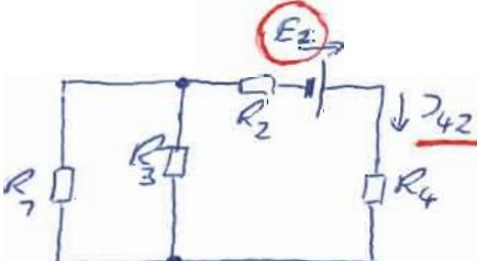
$$\underline{\underline{J_{42} = \frac{E_2}{R_2 + R_4 + \frac{R_1 R_3}{R_1 + R_3}} = \frac{6V}{6\Omega + \frac{72}{7}\Omega}}$$
