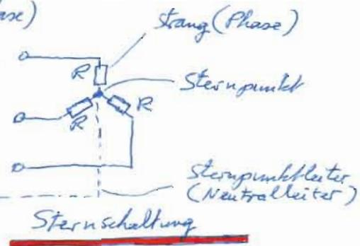
$$\begin{aligned} \text{Leiterspannung } U_{\text{Leiter}} \\ = U_{12} = U_{23} = U_{31} \\ = 400 \text{ V} \end{aligned}$$
