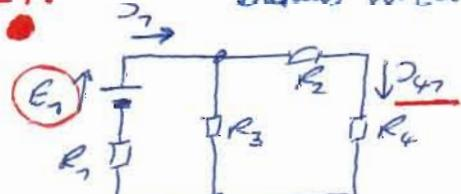
$$J_1 = \frac{E_1}{R_1 + R_3 / (R_2 + R_4)} = \frac{E_1}{R_1 + \frac{R_3(R_2 + R_4)}{R_3 + R_2 + R_4}}$$
