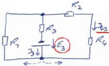
$$\begin{aligned} I_3 &= \frac{E_3}{R_3 + R_7 \parallel (R_2 + R_4)} \\ &= \frac{E_3}{R_3 + \frac{R_7(R_2 + R_4)}{R_7 + R_2 + R_4}} \end{aligned}$$
