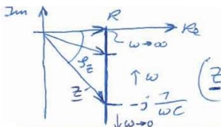
$$\begin{aligned} \underline{Z} &= R + jX \\ &= R + \frac{1}{j\omega C} \\ &= R - j \cdot \frac{1}{\omega C} \end{aligned}$$
