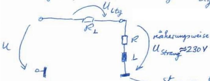
$$\underline{U_{\text{Ltg}}} = \underline{U} - \underline{U_{\text{Strang}}} = R_{\text{L}} \cdot \underline{I}_{\text{Leiter}}$$
