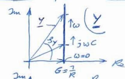
$$\begin{aligned} \underline{Y} &= G + jB \\ &= G + j\omega C \end{aligned}$$
